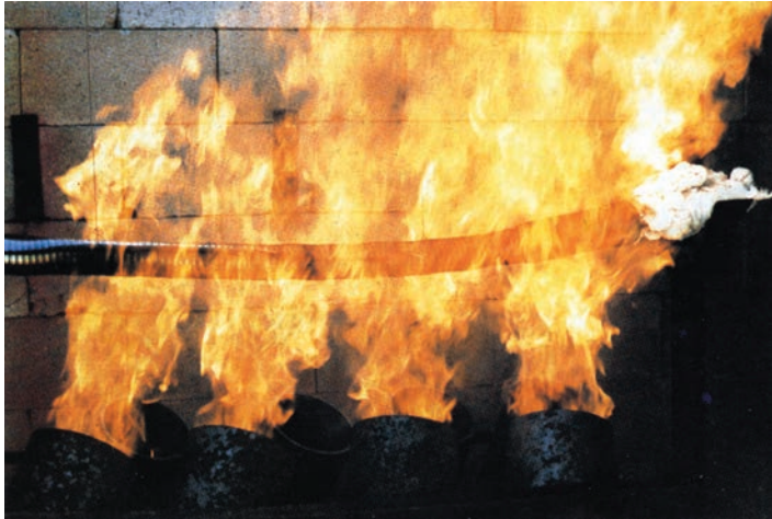
GSM BOP hose tested at 2000°F, 2,000,000 BTU's at 5,000 PSIWP.
